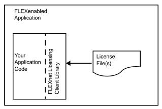
Figure 1-2: FLEXnet Unserved License Component Model
