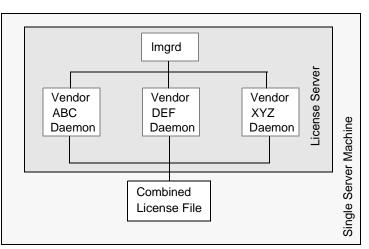
Figure 3-4 shows one possible scenario using a combined license file.
